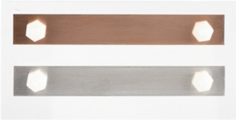
Figure A.6 An alternate design of corrosion classification coupons. Copper and silver metal strips are attached by polytetrafluorethylene fasteners off a plastic plate. The metal strips are unfastened and coulometric reduction analyzed to get the corrosion product thickness.
