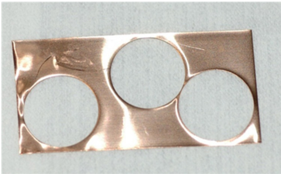
Figure A.4 Coupons, 16 mm (5/8 in.) diameter, are punched out of the 25 x 50 mm (1 x 2 in.) foil exposed for one month in the field. Notice that three coupons can be punched out to make three coulometric reduction runs. Generally, only one or two runs are necessary. The remaining metal foil, as shown above, can be achieved.
