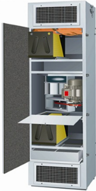
Figure 6.4 Self-contained recirculating air filtration system with (from top to bottom) particulate prefilter, chemical filter, motor blower section, chemical filter, and final filter.
